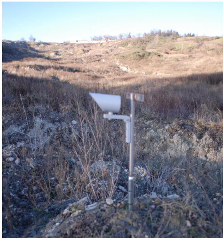
Figure 16. In-field mounting of node support housing a topographic prism.
