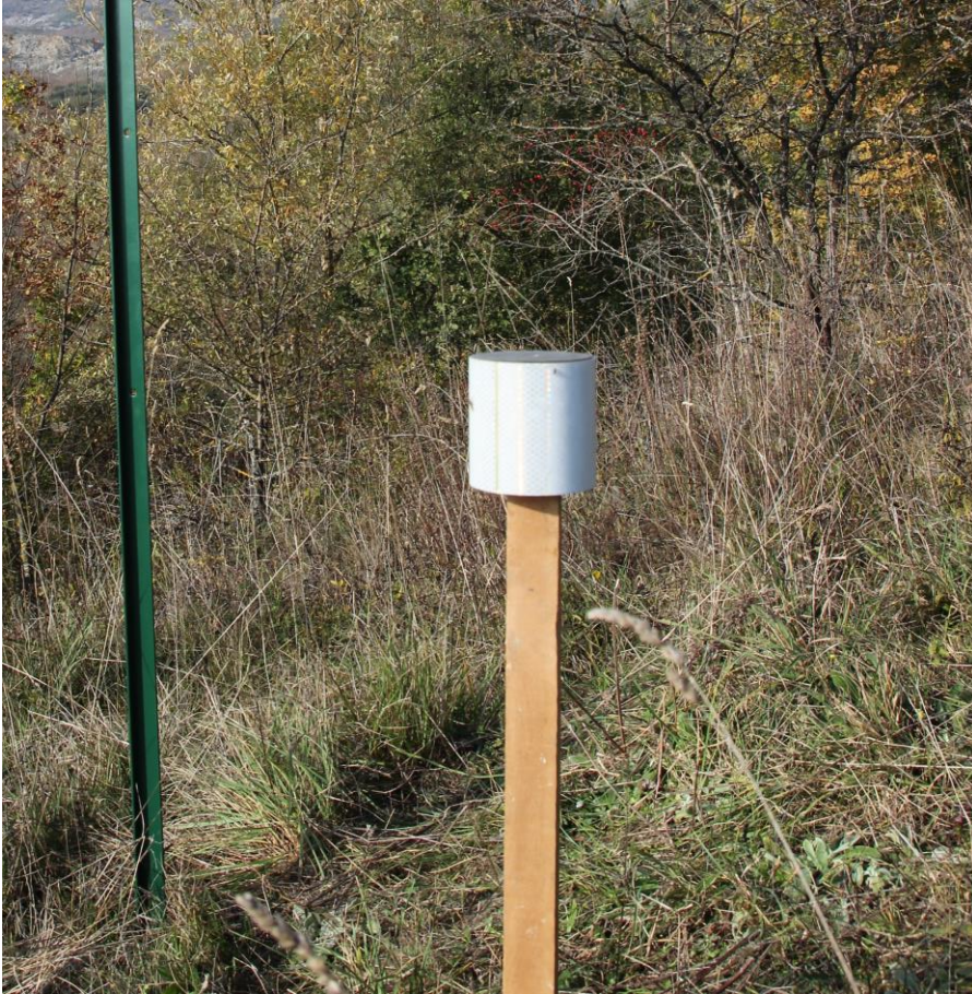
Figure 2. Reference point employed for Terrestrial Laser Scanning data referencing.
