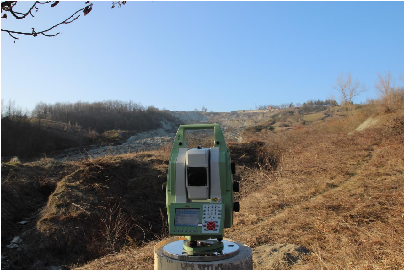
Figure 14. Employed total station device for Roncovetro earthflow traditional monitoring on concrete pillar
